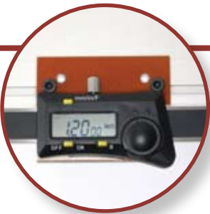
New Digital Scale mounted on WoodRat
